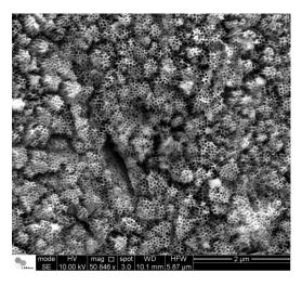
Figure 2. Scanning electron microscope (SEM) micrograph of the Ti specimens after electrochemical anodization treatment
