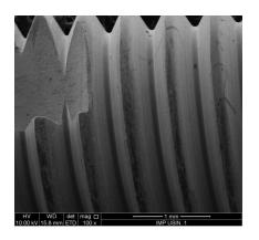
Figure 1. Scanning electron microscope (SEM) micrograph of the anodized implant
